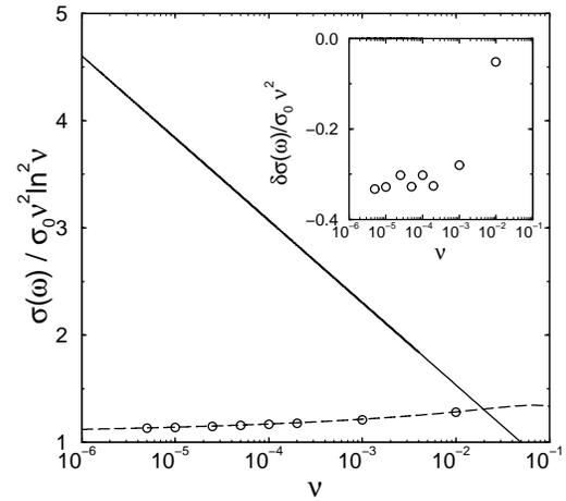
FIG. 1. Dynamical conductivity from solving the Berezinskii recursion equations ( $\nu = 2\omega\tau$ ). Numerical solution ( $\circ$ ), Berezinskii’s solution, eq. (1) (dashed), Gogolin’s result, eq. (2) (solid). Inset: Determining  $C$  by subtracting first three terms in eq. (1) from numerical data:  $C \approx 0.3$ .
